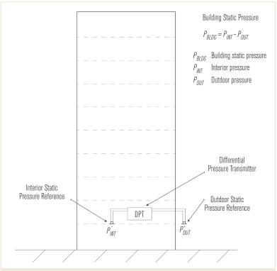
FIGURE 1 Building static pressure measurement with interior and exterior references located at base of building.
