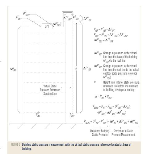
outdoor static pressure reference sensing line, and the change in the virtual outdoor pressure sensing line. Because the exterior section of the outdoor pressure reference sensing line is at the outdoor air temperature, the pressure change within this section of the line will be canceled out by that section of the virtual sensing line, which is above the rooftop penetration of the outdoor static pressure reference sensing line.
