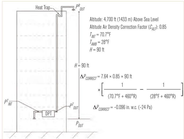
FIGURE 4 Differential pressure transmitter location at the base of building.
