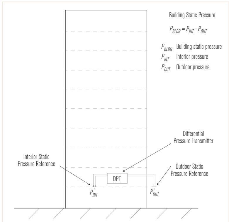
FIGURE 1 Building static pressure measurement with interior and exterior references located at base of building.
