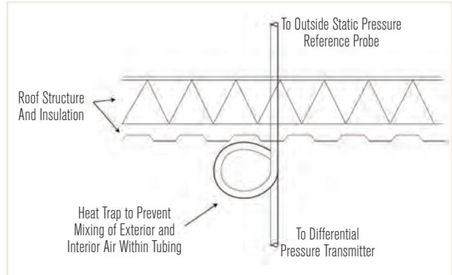
FIGURE 5 Typical heat trap.
