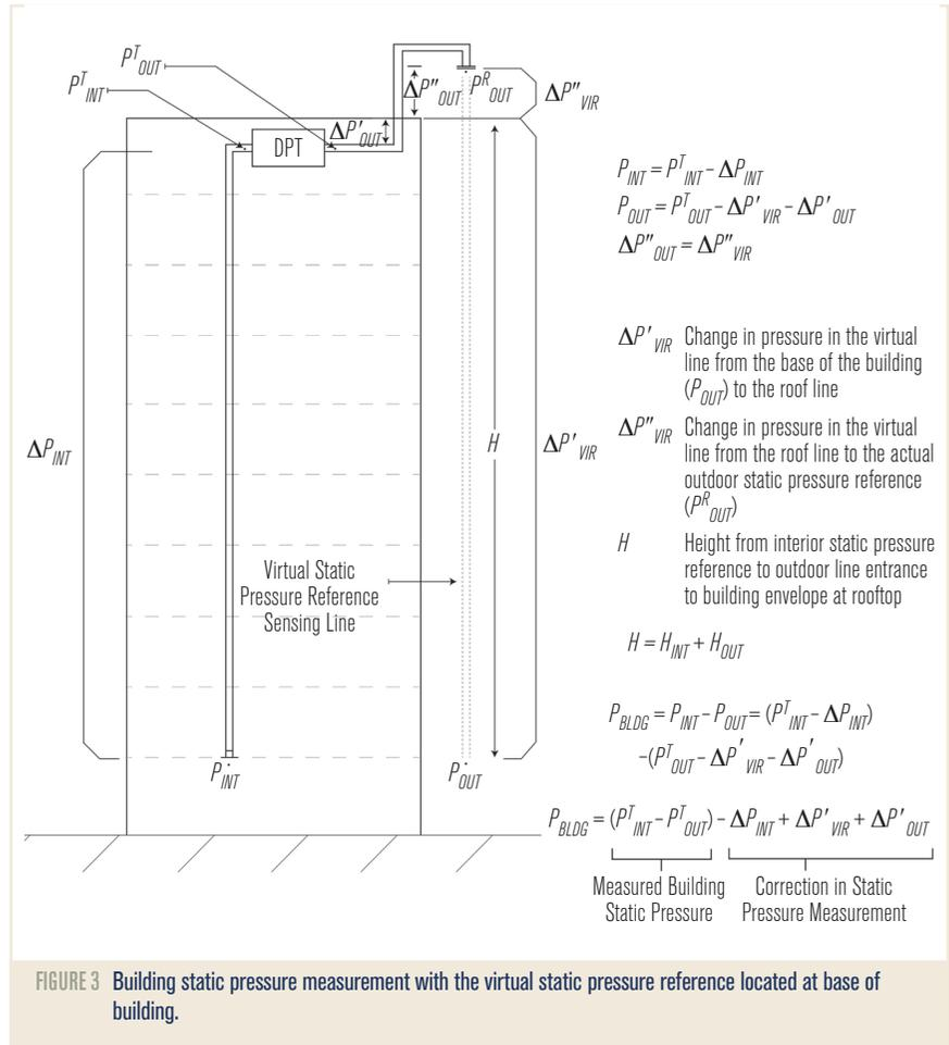
outdoor static pressure reference sensing line, and the change in the virtual outdoor pressure sensing line. Because the exterior section of the outdoor pressure reference sensing line is at the outdoor air temperature, the pressure change within this section of the line will be canceled out by that section of the virtual sensing line, which is above the rooftop penetration of the outdoor static pressure reference sensing line.
