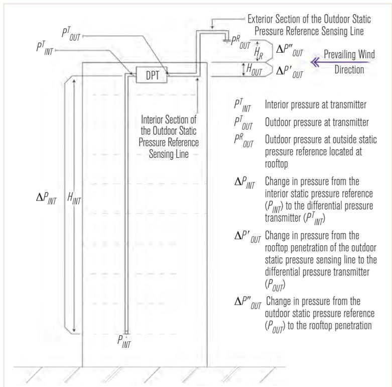
FIGURE 2 Building static pressure measurement with static pressure reference located at the base of building and the exterior static reference located above the roof.
